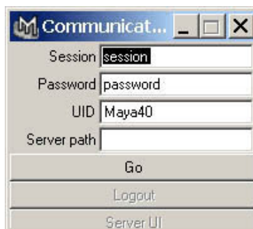
Fig. 3 Dialog box in Maya for setting parameters for session of connection of Maya plugin to communication server.
